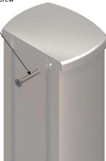
Put lid on, and lock it using a 4,8x32 self-drilling screw
