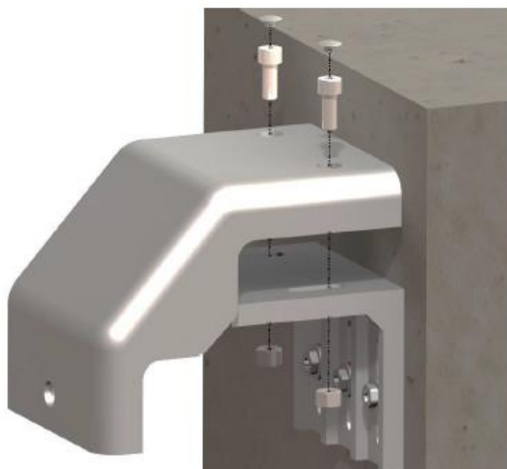
Install angle support using clamp adapted to support
